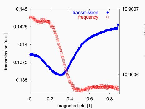
The position of the resonance maximum in transmission and frequency gives the typical CR
