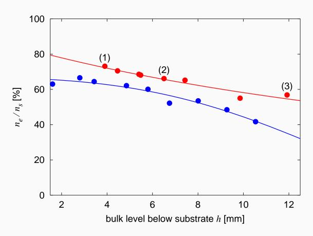
Fit of the model parameters of the localized electrons to the data. From the data on PMMA we get  $\Delta$  around 8 nm and η around 6 nm. These values, being in the nm-regime, are reasonable and typical for the surfaces used in the experiments.
