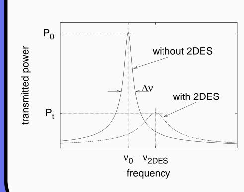
The dependence of the resonance of the cavity with and without a 2DES on the helium film on the substrate is shown.
